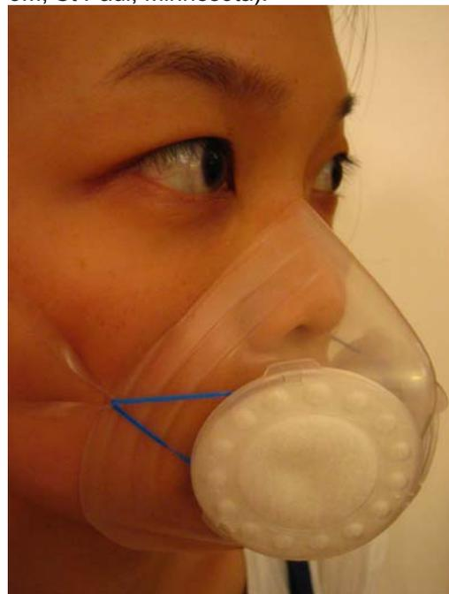
Figure 1. Totobobo mask. Inspired gas is filtered by HEPA filters. Plastic can be cut to fit wearer's face. Transparency allows observation of contact between the plastic and the wearer's face.
